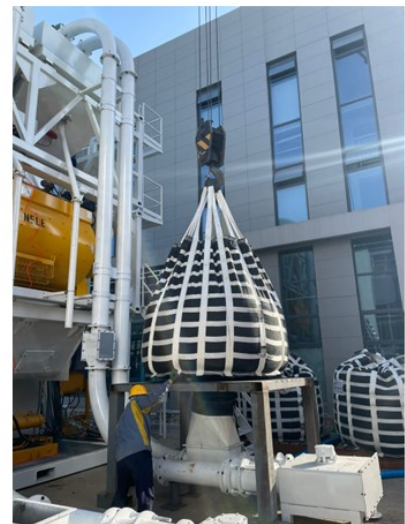
The CPT45 spread using high density grout material and 8.5 MT UFIC bags.
